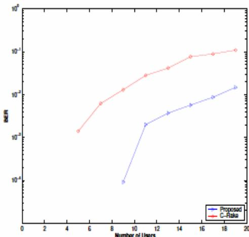
Fig 2: BER vs. No. of users for CM1 with  $E_b/N_0 = 20$  dB
