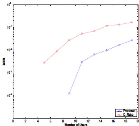
Fig 3: BER vs. No. of users for CM2 with  $E_b/N_0 = 20$  dB
