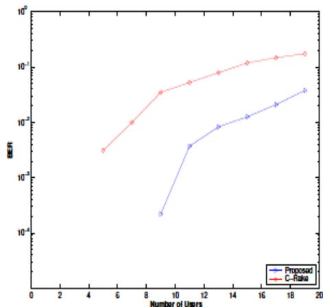
Fig 4: BER vs. No. of users for CM3 with  $E_b/N_0 = 20$  dB
